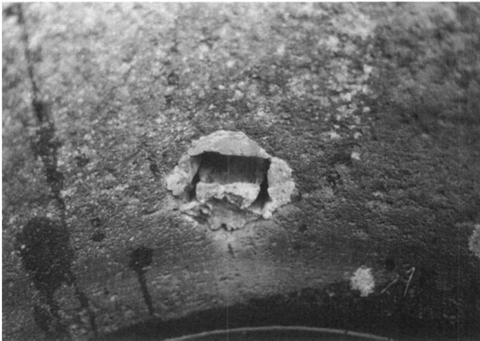
42. A hole with lead in the inner side of a kneading-machine. A wooden blade was attached in the hole.
